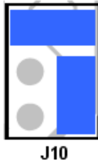
Figure 7 J10 Jumper settings for Current output
