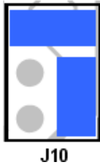
Figure 7 J10 Jumper settings for Current output
